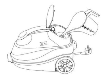
Fill the boiler with at least 500ml of water. In order to get dry steam, fill the boiler to the maximum (2000 ml). Overfill water will bring water in the steam.
